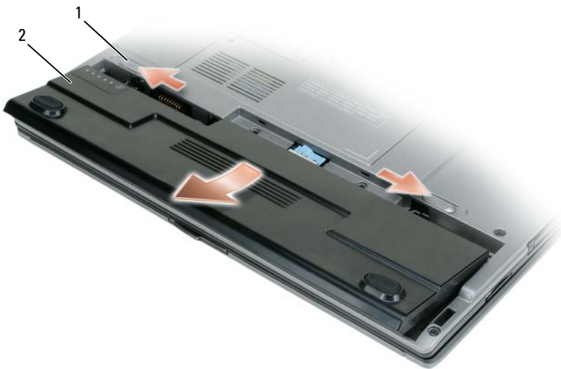
1 battery-bay release latch (2) battery
